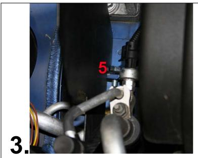
Mount the heat shield in the original holdings (5) and (6 pic 4.) Use M8 screw, nut and washer. First fasten the shield to the lower holding (5). Do not tighten fully yet.
