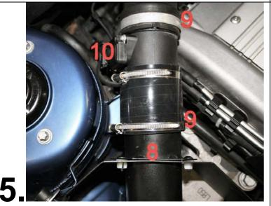
Mount the air pipe to the heat shield. (With the flang 8 on the outside of the shield as picture shows.) Use screw (3psc)
