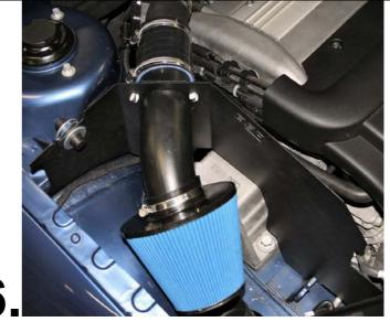
Mount the air filter and tighten the hose clamp.
