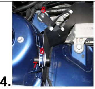
Now fasten the shield in the rear holdings (6) Use 1 rubber washer and 2 steel washer to each holding. Make sure the shield is correctly fitted, then tighten all the loose screws.
